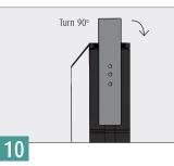
Attach the feet, by mounting them following the module length as if they are folded into the bottom of the frame, afterwards turn your feet 90 degrees to point out from the banner.
