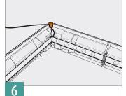
Insert the electric wire, and lead it through the small opening at the orange corner module.
