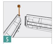
Pull up the orange plug and attach the two sides in the orange corner area to each other. Afterwards then push the orange plug back down to lock the two sides together.
